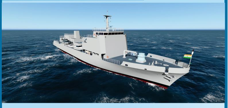
The Contract for the four-ship Survey Vessel (Large) project was signed on 30 Oct 2018. These ships are capable of full scale coastal & deep-water hydrographic survey of Ports & Harbors, as well as of approaches & determination of navigational channels & routes. In addition, the ships are also capable of undertaking survey of maritime limits and collection of oceanographic & geographical data for Defence applications.
